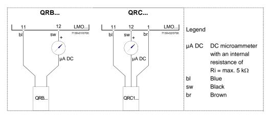
As an alternative to detector current measurement, the diagnostic tool OCI400 / with PC software ACS400 / ACS410 can be used. In that case, the DC microammeter is not required.
