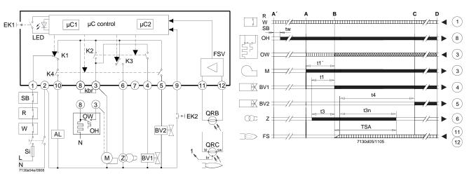
AL Alarm device BV... Fuel valve
