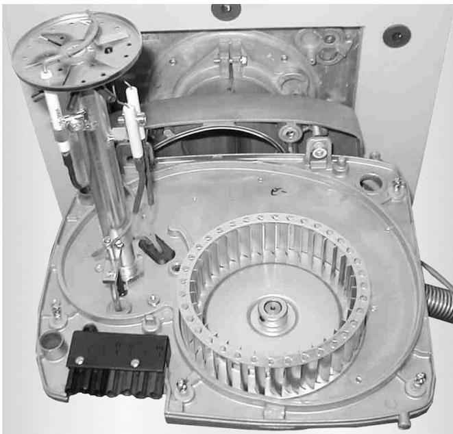
Abb. 18: Serviceposition SGN ...H
