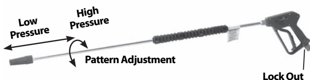
Figure 17 – Wash Wand Nozzle Adjustments
