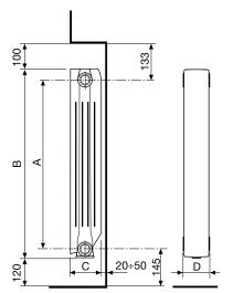
**STANDARD SUPPLY:** Available from 3 to 10 sections for centre distance 800 – from 3 to 12 sections for centre distance 700 - from 3 to 14 sections for centre distance 350-500-600.
