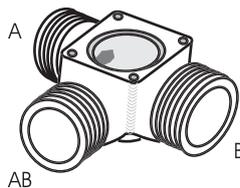
Outer and inner thread on all three connections (A, B, AB)
