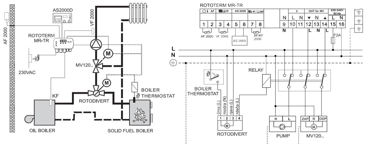
Diverter valve switches between two heating sources. This combination ensures utilisation of cheaper energy source. When this source is consumed, reversible valve switches to the second energy source and with limit switches, which are in the actuator, activates the second energy source. For heating regulation is used regulator ROTOTERM MR-TR.
