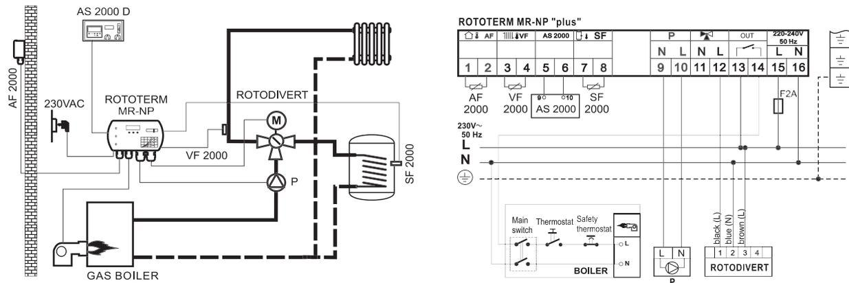
In combination with "ROTOTERM MR-NP" automatic control system of the house this separating valve enables heating of a residential unit and sanitary water with just one pump, where sanitary water has priority. The flow through the pump is never completely closed by ROTODIVERT diverter valve, therefore no pressure shocks appear.
