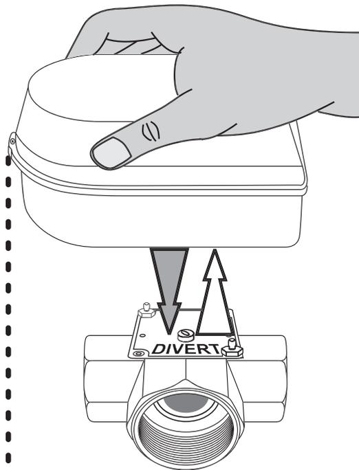
M4 screw is inserted at the bottom of the actuator and prevents removal of the actuator from the valve by unauthorised person
