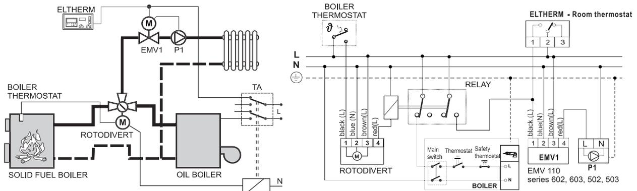
Diverter valve switches between two heating sources. This combination ensures utilisation of cheaper energy source. When this source is consumed, reversible valve switches to the second energy source and with limit switches, which are in the actuator, activates the second energy source. The flow through the pump is never completely closed by F3L reversible valve, therefore no pressure shocks appear.
