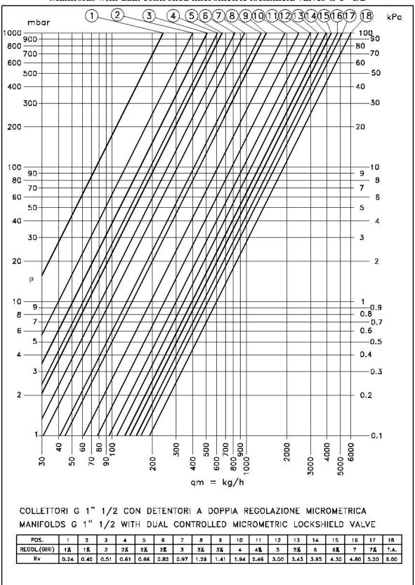
Manifolds with dual controlled micrometric lockshield valves G 1" 1/2
