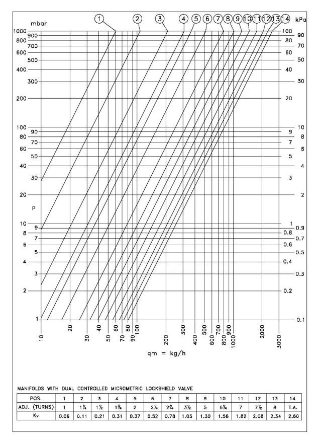
Manifolds with dual controlled micrometric lockshield valves G 1" - G 1" 1/4
