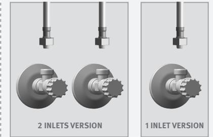
**MAKE SURE THAT THE FILTERS ARE INSTALLED BETWEEN THE FLEXIBLE PIPE AND THE SHUT OFF VALVE/ANGLE VALVE (NOT SUPPLIED).**
