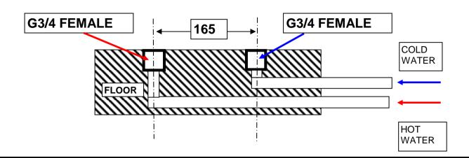
SCREW THE 2 TUBES ON THE 2 FLOOR CONNECTIONS **G3/4 FEMALE**, WITH THE WALL FLANGES ALREADY SCREWED AND SOME TEFLON TAPE ON THE THREADS TO SEAL THEM
