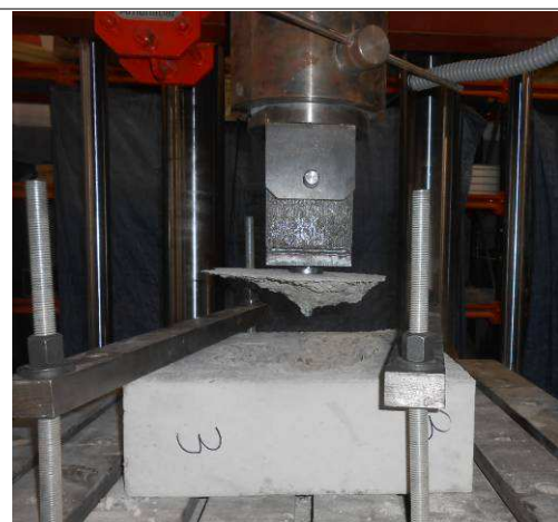
DNBOLT 16L: Breakage of test member (cone) Sample nº3
