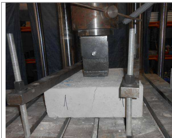
DNBOLT 16L: Breakage of test member Samples nº 1, 2, 4, 5 y 6
