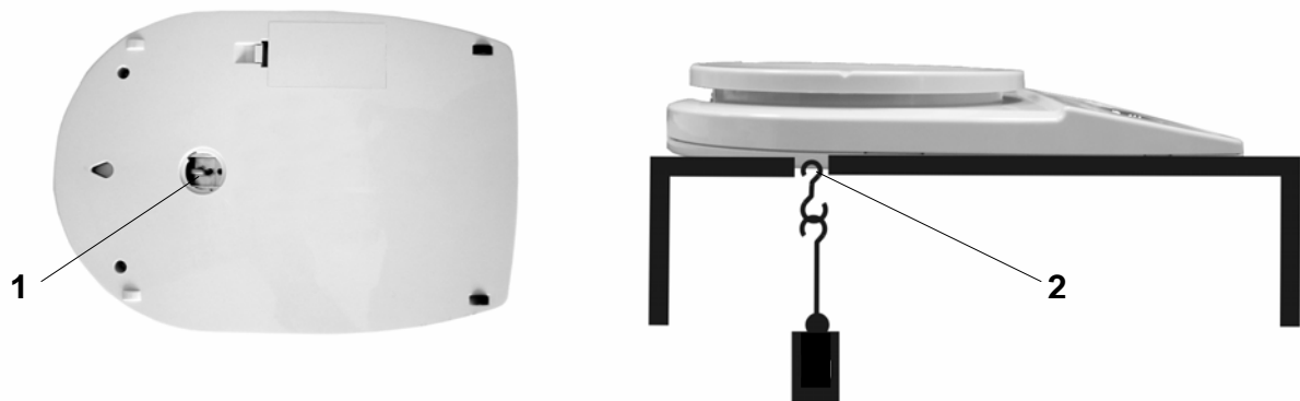
Fig. 1: Setting up the balance for underfloor weighings
