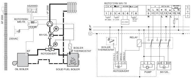
Diverter valve switches between two heating sources. This combination ensures utilisation of cheaper energy source. When this source is consumed, reversible valve switches to the second energy source and with limit switches, which are in the actuator, activates the second energy source. For heating regulation is used regulator ROTOTERM MR-TR.
