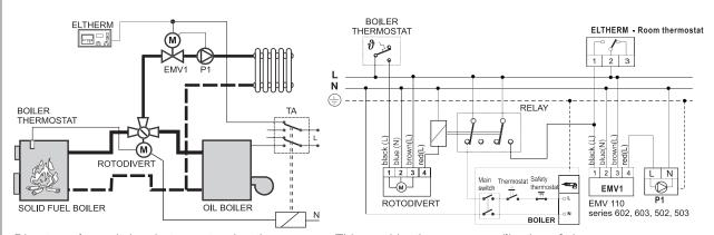
Diverter valve switches between two heating sources. This combination ensures utilisation of cheaper energy source. When this source is consumed, reversible valve switches to the second energy source and with limit switches, which are in the actuator, activates the second energy source. The flow through the pump is never completely closed by F3L reversible valve, therefore no pressure shocks appear.
