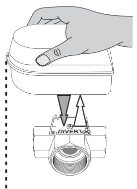
M4 screw is inserted at the bottom of the actuator and prevents removal of the actuator from the valve by unauthorised person
