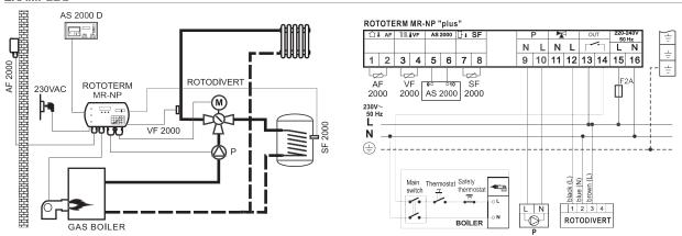
In combination with "ROTOTERM MR-NP" automatic control system of the house this separating valve enables heating of a residential unit and sanitary water with just one pump, where sanitary water has priority. The flow through the pump is never completely closed by ROTODIVERT diverter valve, therefore no pressure shocks appear.
