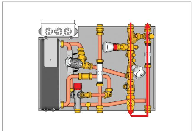
Figure 6 – Heating function – primary side
