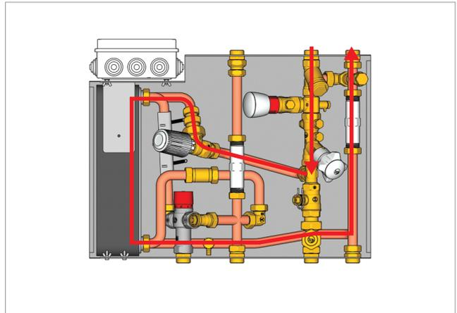
Figure 8 – Sanitary hot water function – primary side
