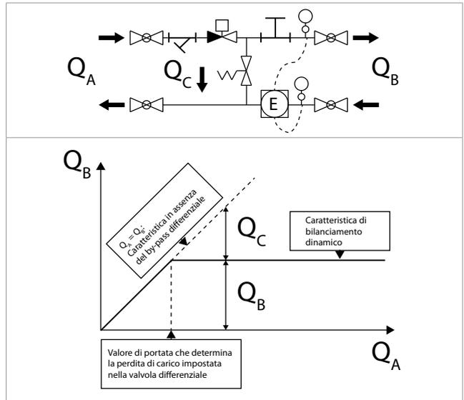
Figure 4 – Operating characteristic of the dynamic balancing
