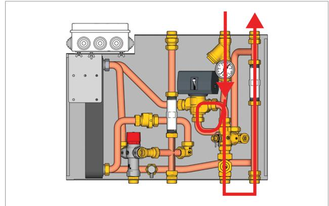
Figure 5 – Heating function – primary side
