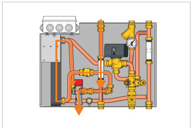
Figure 13 – Sanitary hot water (SHW)
