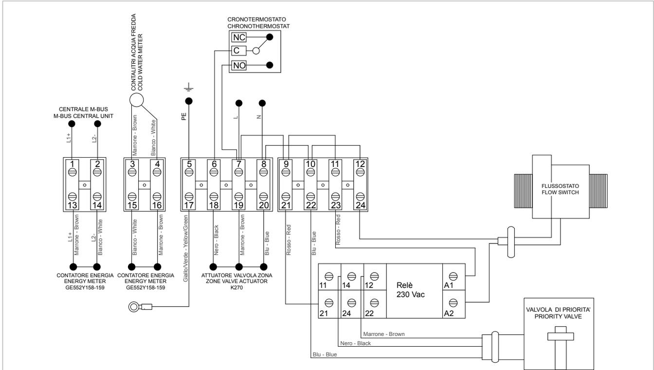
Figure 18 - Electric connections of the terminal board
