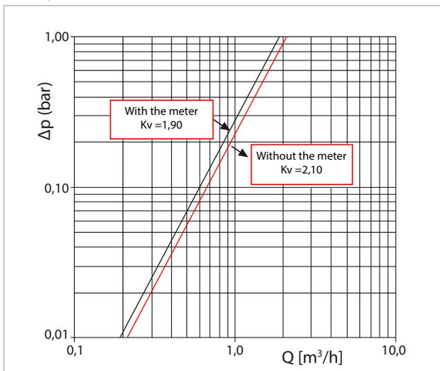
Figure 5 – Heating function – primary side
