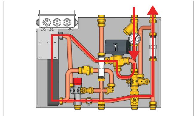
Figure 7 – Sanitary hot water function – primary side
