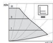
Recommended for underfloor heating or for large-sized pipes, applications without a variable pipe network curve (e.g. storage charge pumps) or single-pipe heating systems with radiators.
